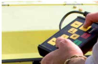
Cable remote with flexible spiral cable
