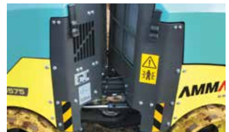
Maintenance-free articulation joint with oscillation for perfect ground contact
