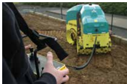
Additional cable connection as standard
