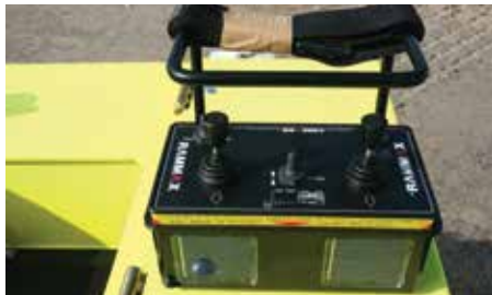
IR transmitter with solar panels
