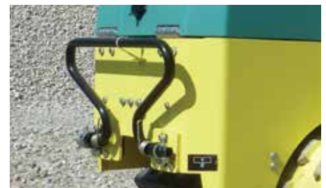
Optional safety bar with simple transport lock
