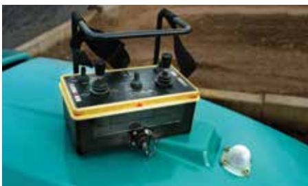
Infrared remote control with solar panels – No charging on the mains. Automatic charging during work
